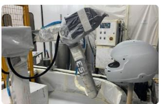
Plant with **Lesta LEBOT WP** mounted on a small mobile conveyor with integrated panel. The robot is configurated to repeat a continuous movement
